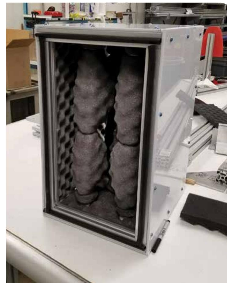
**Talmadge's original idea was to line a box with shipping foam. I added baffles with PVC pipe wrapped in the foam. We ran with it, and it worked astonishingly well.**
