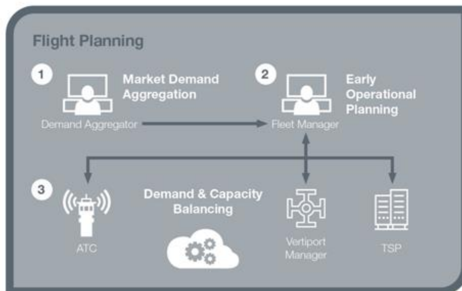
Figure 12. Flight Scheduling Sequence and Flow
